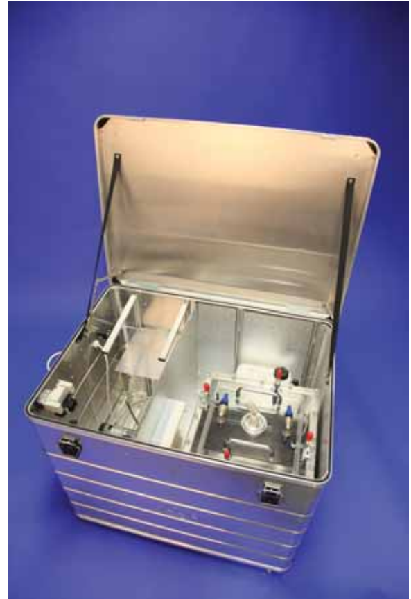
Fig. 1: Mobile Circulatory Module (mCM) housing for ex-vivo lung perfusion
