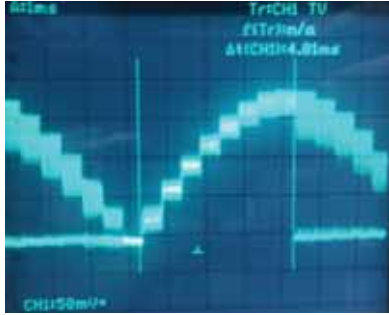
Fig 2: Voltage curve of stepper motors with rectangular steps in form of a sine wave.
