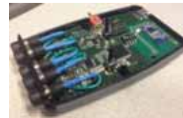
Fig. 2: EEG amplifier circuit board mounted in the HAMMOND housing.
