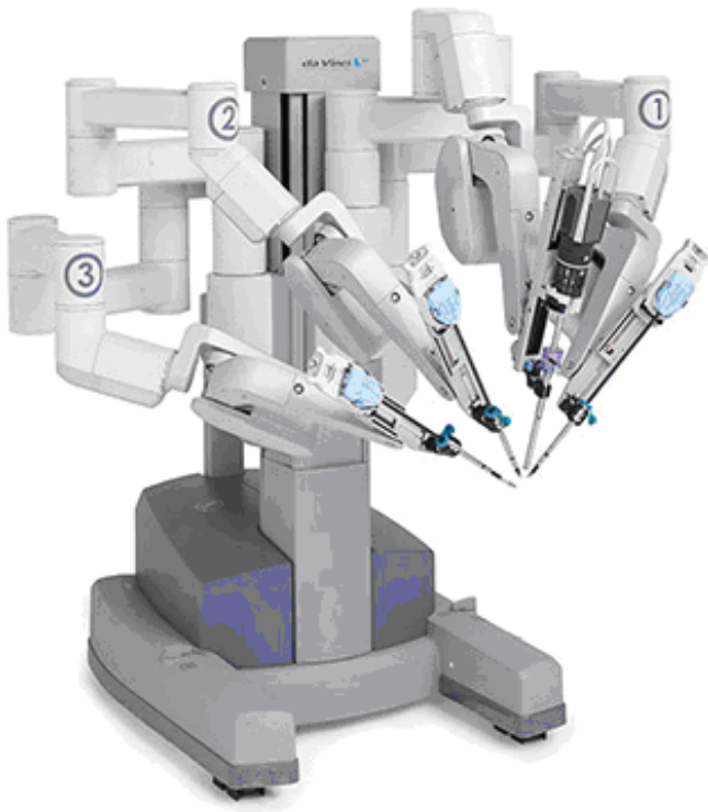
Fig 1: DaVinci surgery robotics, each surgery tool can precisely be controlled in many degrees of freedom [1].
