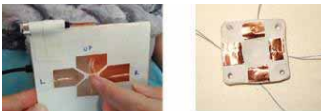
Fig 2: Capacitive model, left first prototype, right improved prototype.
