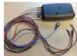
Fig. 4: Measurement setup for two channel EEG measurement (green – CH1+, red – CH1-, blue – Ch2+, brown – CH2-, gray – RLD).
