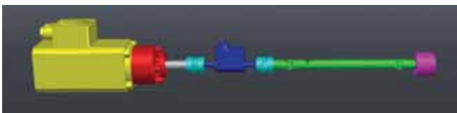
Fig 2: Internal structure of the test station including motor (yellow), gear box (red), couplings (cyan) and sensor (blue) and shaft to the ergometer (green).
