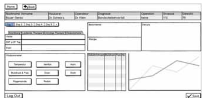
Fig 1: Application mockup showing the display of the vital parameters which can be changed by buttons including a table and additional graph for a better overview.
