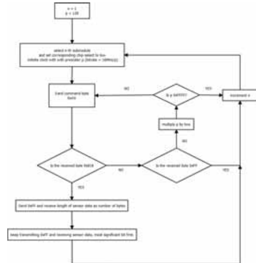
Fig. 2: Simplified flow diagram of slave discovery and support for variable SPI clock speed.
