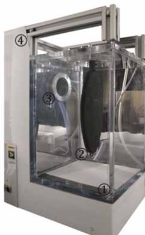
Figure 1: Representation of the i-Lung model. (1) PMMA chamber, (2) Latex bag, (3) piston system enabling the pressure variation within the chamber, (4) movable setup.
