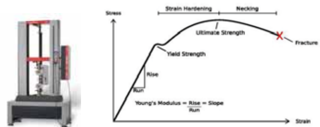
Figure 1: Industrial tensile test machine (left)[4] and stress–strain curve (right).[5]
