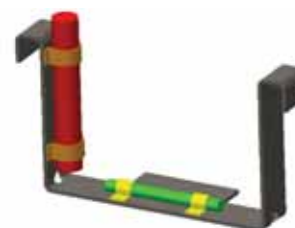
Figure 1: The sensor (green part) and heating element (red part) placement on the designed stainless steel plate.
